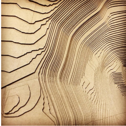
Layered Site Model using Contour Method (Example)
